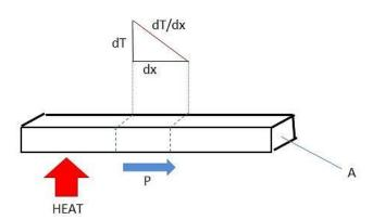
Let us assume **the ideal condition** that the sides of the bar are fully insulated so that no heat is exchanged between the sides and the surroundings.
