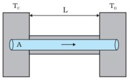
Consider a metallic bar of length L and uniform cross section A with its two ends maintained at different temperatures. (Note the length inside the chambers is ignored). This can be done, for example, by putting the ends in thermal contact with large reservoirs at temperatures, say,  $T_C$  and  $T_D$  respectively **Steady state heat flow** by conduction in a bar with its two ends maintained at temperatures  $T_C$  and  $T_D$ ; ( $T_C > T_D$ ).
